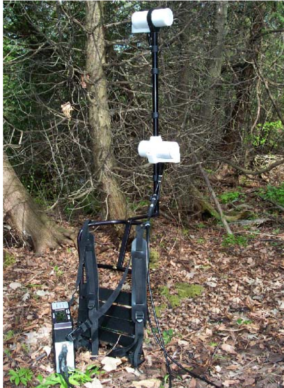
Figure 4: Gradiometer and Backpack Assembly
